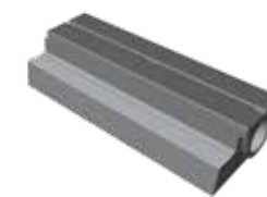
BODAN S-BORD - Edge beam with integrated slit drainage gutter - Prevents soiling of the track ballast and moisture penetration of the track bed - Resistant to frost and de-icing salt - High slip resistance thanks to the rough grain surface - Made of polymer concrete
